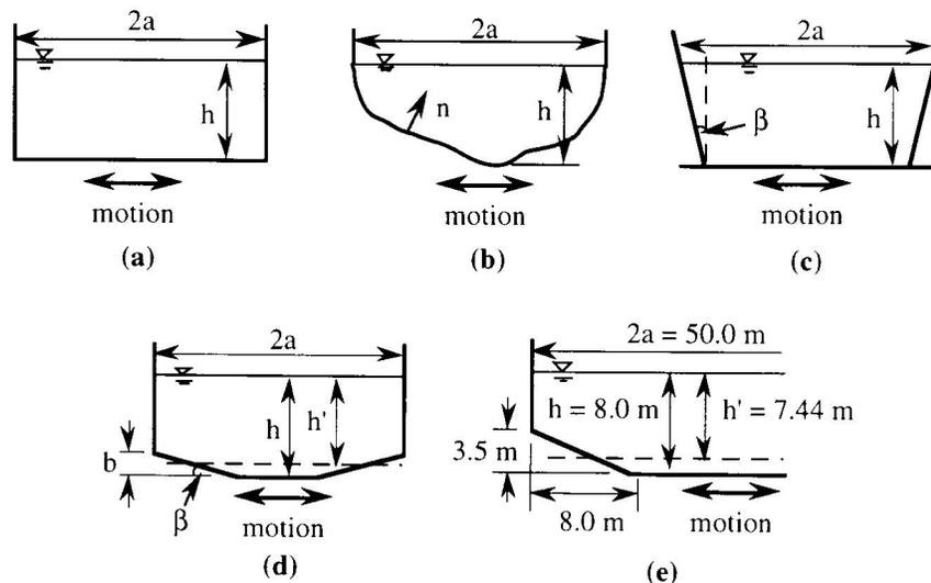
Fig. 1. Definition sketches. (a) rectangular reservoir, (b) reservoir with arbitrary section, (c) reservoir with steep sides, (d) reservoir with sloping floors, (e) example reservoir.
