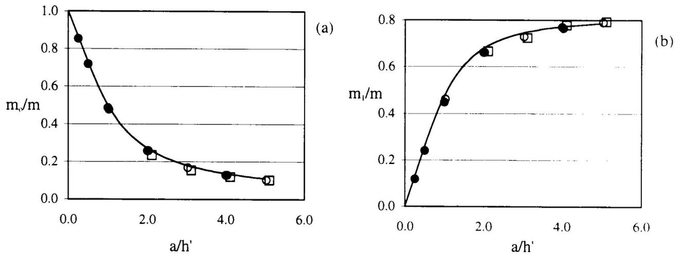
Fig. 3. Relative masses  $m_0/m$  and  $m_1/m$  as functions of relative reservoir size  $a/h'$  for a rectangular reservoir with various floor slopes  $\beta$  and relative floor elevations  $b/h$ . —, closed-form solution for  $\beta = 0^\circ$ ,  $b/h = 0$ ; numerical model: ●,  $\beta = 0^\circ$ ,  $b/h = 0$ ; ○,  $\beta = 10^\circ$ ,  $b/h = 0.1$ ; □,  $\beta = 10^\circ$ ,  $b/h = 0.2$ . (a)  $m_0/m$ , (b)  $m_1/m$ .
