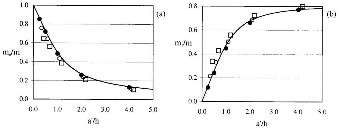
Fig. 2. Relative masses  $m_0/m$  and  $m_1/m$  as functions of relative reservoir size  $a/h$  for a rectangular reservoir with various side slopes  $\beta$ . —, closed-form solution for  $\beta = 0^\circ$ ; numerical model: ●,  $\beta = 0^\circ$ ; ○,  $\beta = 10^\circ$ ; □,  $\beta = 20^\circ$ . (a)  $m_0/m$ , (b)  $m_1/m$ .
